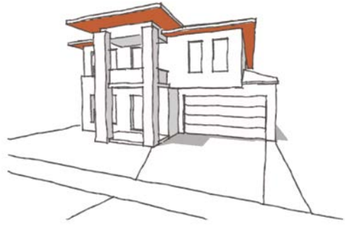
Diagram 2.7.1.4: Minimum 450mm eaves on second storey
