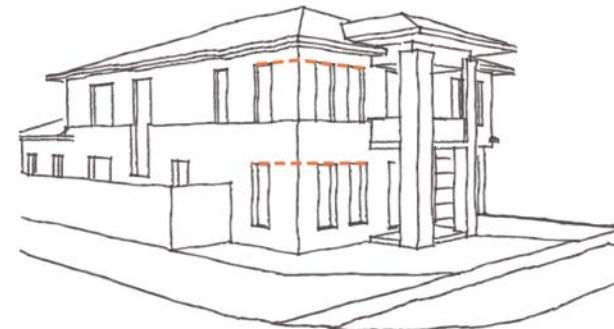
Diagram 2.8.2.1: Matching window head height on front and side façades
