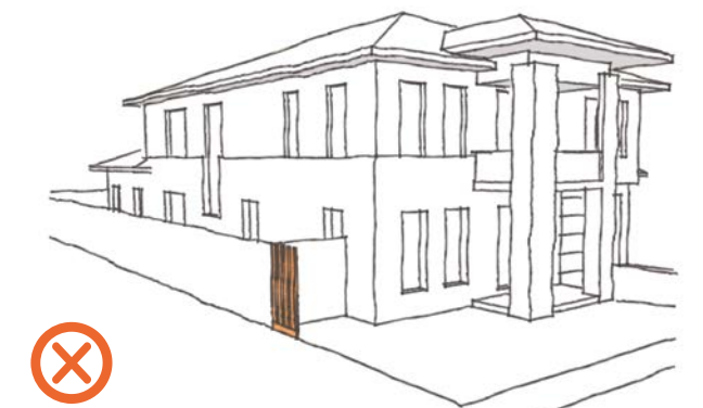
Diagram 3.2.7.4: Side fences should not extend beyond the return fence
