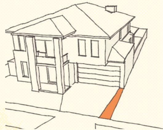
Diagram 3.1.3: Driveways should be set back a minimum 0.5m from side boundary
