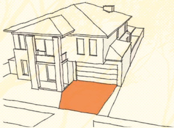
Diagram 3.1.2: Driveways should match the width of garage opening and the crossover
