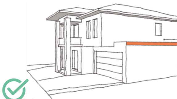
Diagram 2.7.3: Parapet must return at least 500mm
